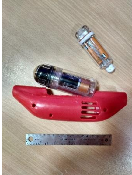
Figure 24. Low-cost, low profile LED lights and acoustic alarms (pingers) developed by Fishtek Marine.
